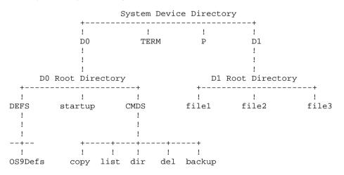
The device names in this example system are "TERM", "P", "D0" and "D1". The root directory of device "D0" includes two directory files, DEFS and CMDS, and one ordinary file "startup". Notice that device "D1" has in its root directory three ordinary files. In order to access the file "file2" on device "d1", a pathlist having two names must be used:
